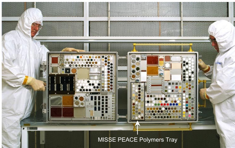
Figure 4. MISSE PEC 2 with Tray 1 on the right and Tray 2 on the left. 18
